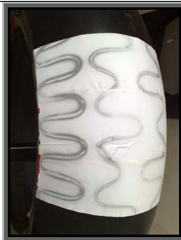
Pic 6: Heating wires in waves
