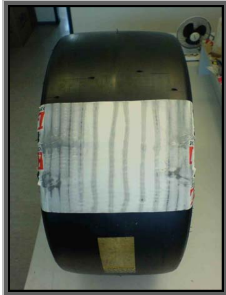
Pic 2: Racing car tyre, heated with conventional hot wire technology
