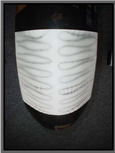
Pic 3: Thermographic result on a motorcycle tyre with conventional tyrewarmer . . .
